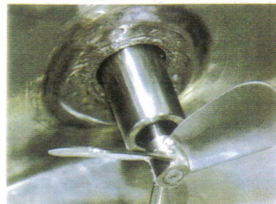
7. Sealed-off apertures for rotating parts, whereby the exchange of contaminated material with the neighbouring space and the wear and tear of the sealing material is markedly heavier (e.g. stirrers).
