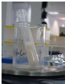
Weigh 1g of homogenous sample
